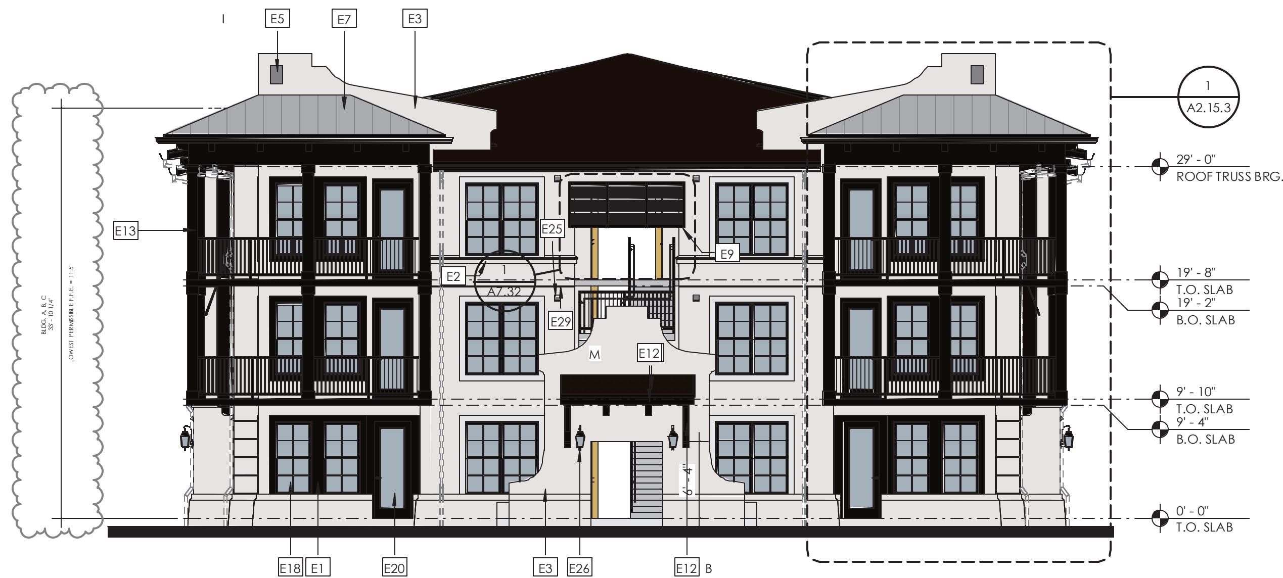
2 BLDG TYPE 15 - LEFT ELEVATION
