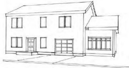
A garage door no wider than 30 percent of the width of the front wall plane will maintain an acceptable scale along the street front.
