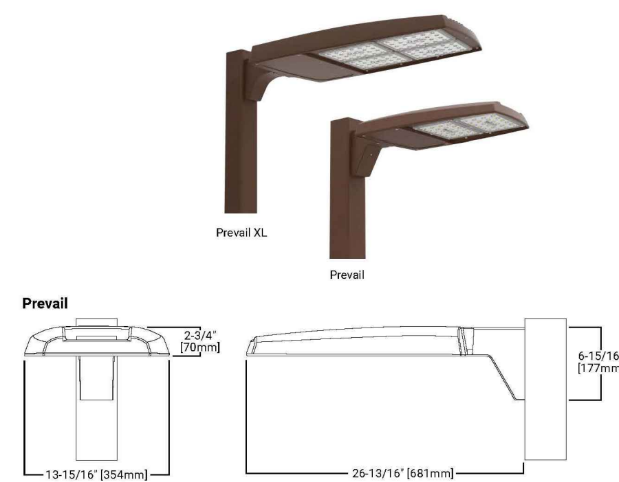
VALMONT STRUCTURES, INC. DIRECT BURIAL CONCRETE POLE PARKING LOT LIGHTING FIXTURE TO BE USED ON ALL PARKING LOT LIGHTING (20' MOUNTING HEIGHT) N.T.S.
