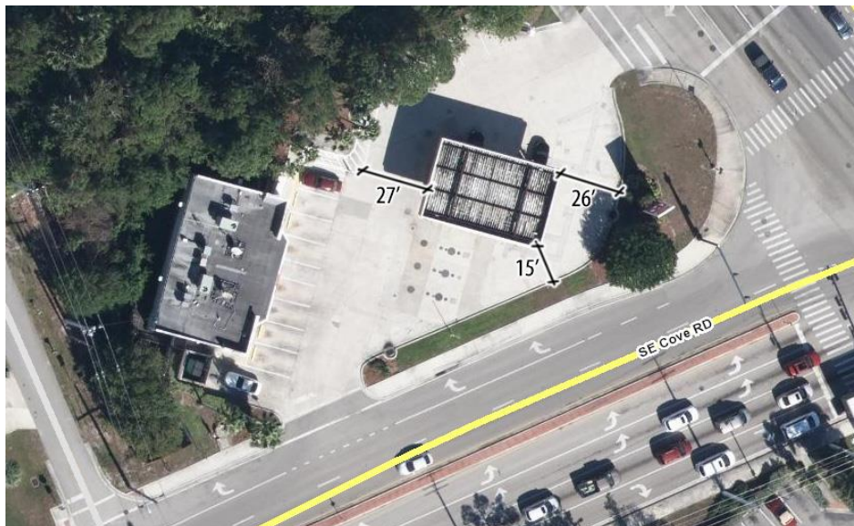
Exhibit 7: Aerial of the current gas station located on the property. The narrow drive aisles can be seen clearly. (This design does not work, traffic builds up around the entrances, and customers complain). This property is located along the primary North-South travel route East of I-95, and a primary East-West travel route leading to I-95.
