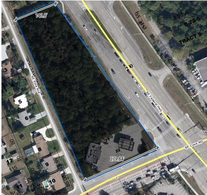
Exhibit 6: Uniquely Situated along three (3) Martin County roadways, the property shape does not allow parallel offsets because it creates pinch points. Southern Property line- 279.84 feet, Northern Property line- 146.8 feet.
