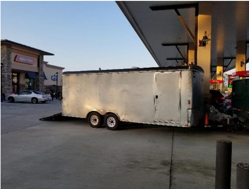
Photograph 2: An example of a large Lawn Maintenance Vehicle and trailer at a fuel pump. (Without the larger drive aisle, the trailer would encroach into the drive aisle posing a safety hazard and the cars parked in front of the store would be unable to back out safely.)
