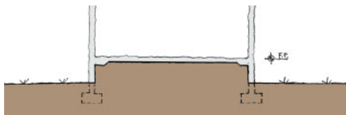
Stem Wall, Extended Footers or Thickened Monolithic Foundation with Fill
