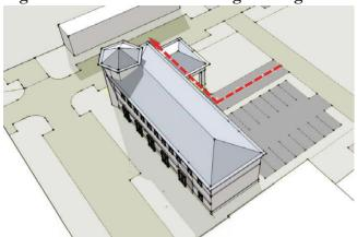
Drive through stacking occurs in the rear of the lot. Circulation is from the alley, exiting to a secondary street.
