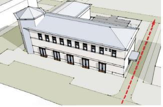
Circulation and stacking occurs along the side of the building. Cars enter from the alley and exit onto the street.
