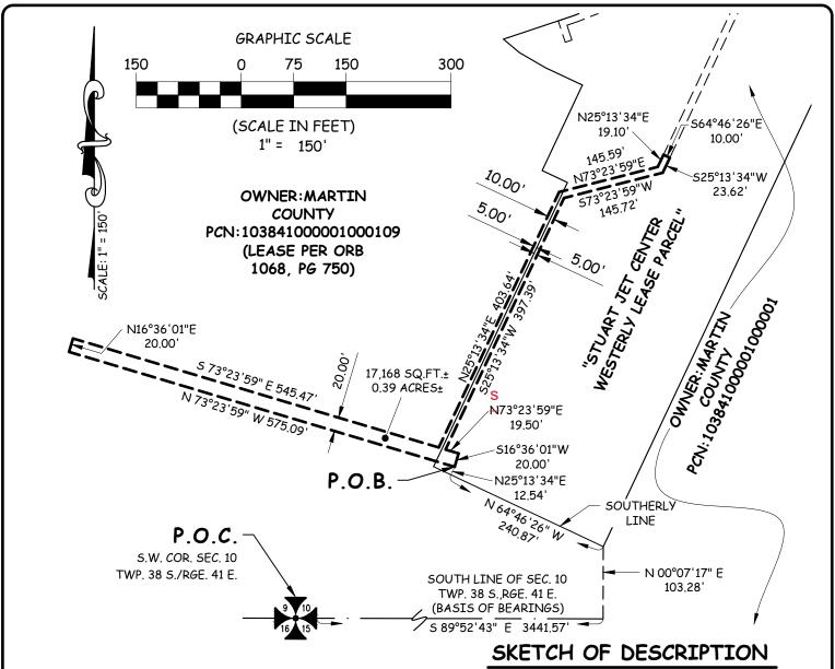
BEARINGS SHOWN HEREON ARE REFERENCED TO THE SOUTH LINE OF SECTION 10, TOWNSHIP 38 SOUTH, RANGE 41 EAST, HAVING A ASSUMED BEARING OF S 89°52'43" E, ALL OTHER BEARINGS ARE RELATIVE THERETO.
