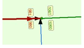
**RCL Address Range Overlap** — Code 503 An address should only appear one time in the RCL feature class. Adjoining, contiguous segments are checked to ensure that address ranges do not overlap between them.
