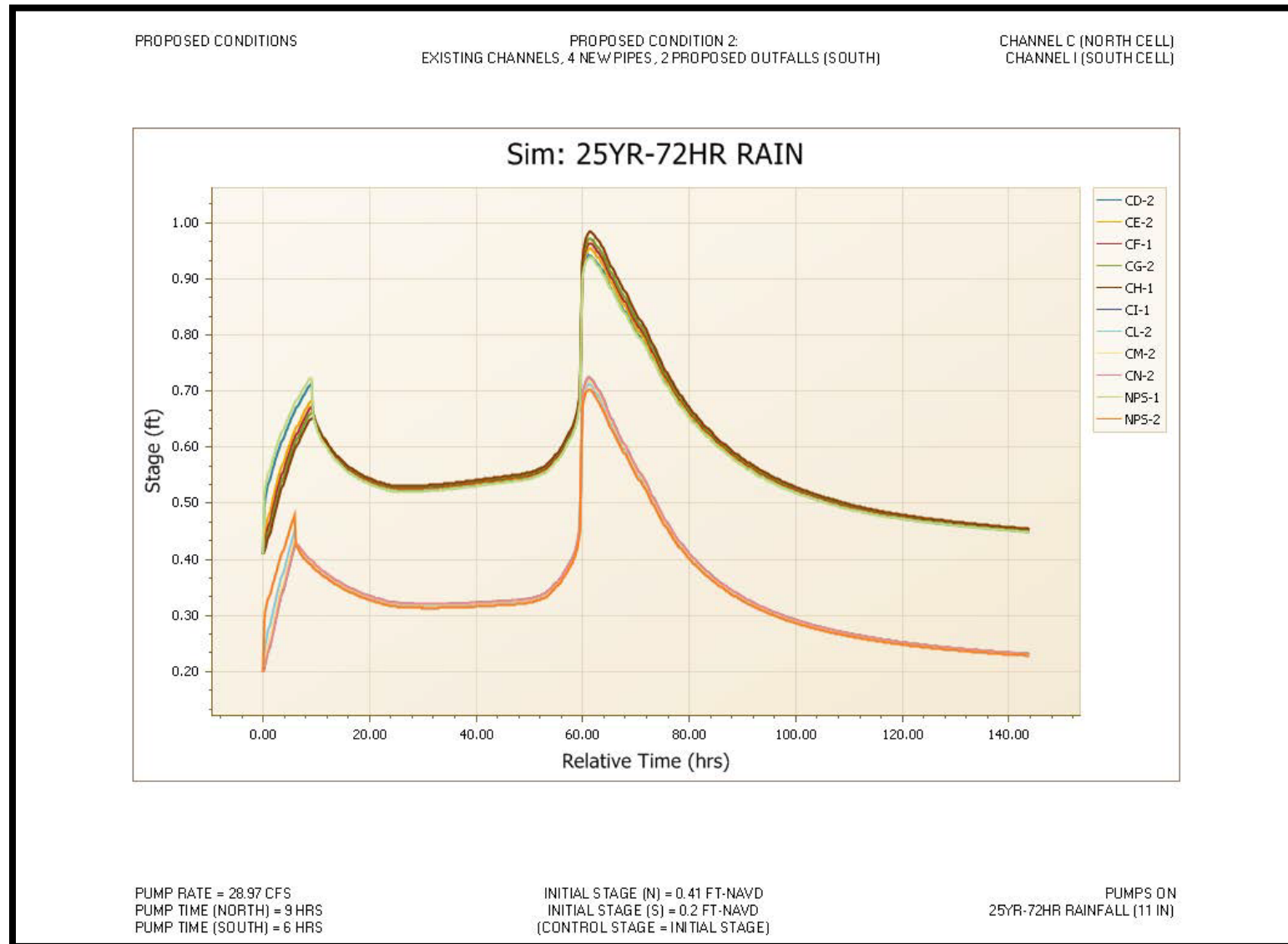
Figure 21. Proposed Condition 2: Time versus Stage graph for Channels C & I, Pumping plus 25-year, 72-hour storm event scenario
