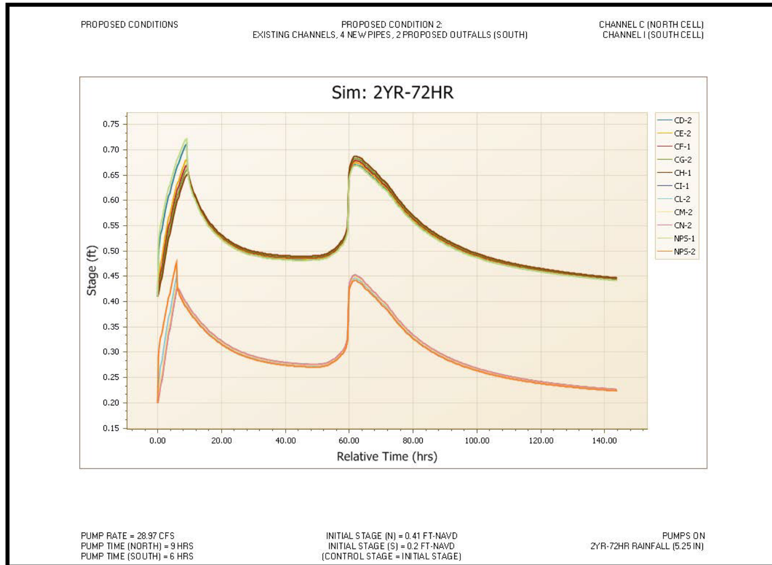
Figure 22. Proposed Condition 2: Time versus Stage graph for Channels C & I, Pumping plus 2-year, 72-hour storm event scenario
