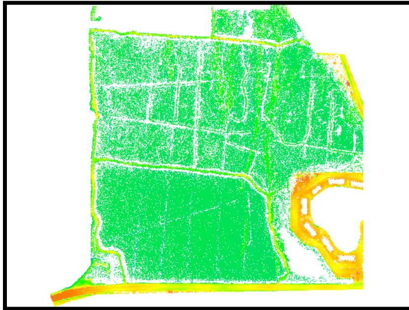
Figure 4. LiDAR Points Imported & Aggregated as 3'x3' Raster Grid
