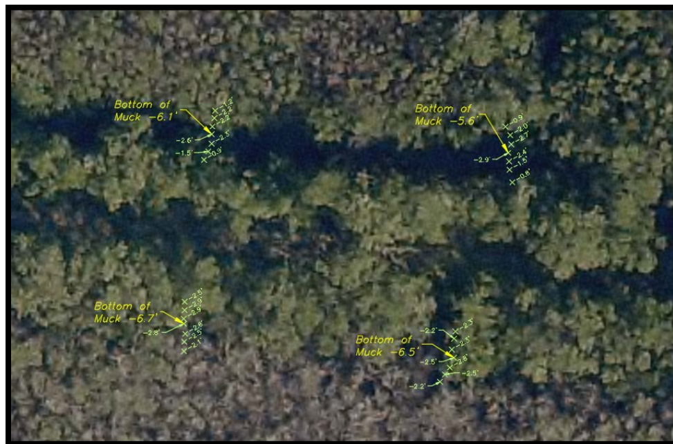
Figure 2. Examples of surveyed channel cross-sections, parallel to central access berm
